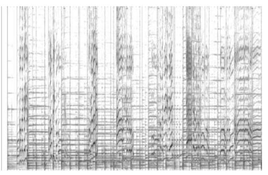
Spectrogram up to 0:40, 10 Hz to 5 kHz, window size 4096 samples
