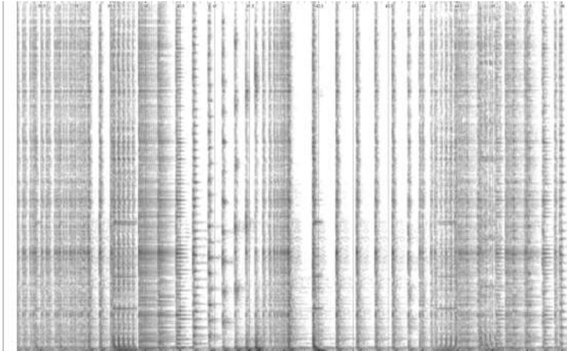
Spectrogram 0:38 - 0:46, 10 Hz to 10 kHz, window size 4096 samples
