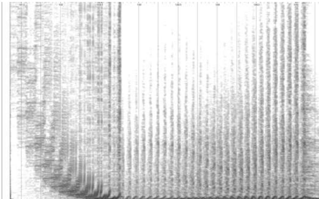
Spectrogram 1:01 - 1:05, 10 Hz to 10 kHz, window size 4096 samples
